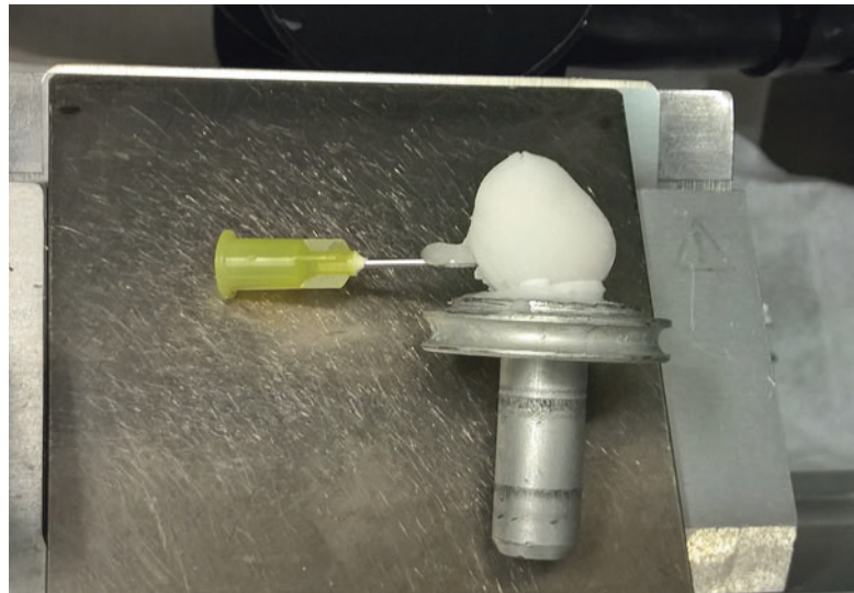
Fig. 3 Image of CMC embedded mouse eye attached to a cryostat chuck with the mark on the luer lock of the needle oriented toward the chuck and mounted with the needle parallel to the chuck surface
